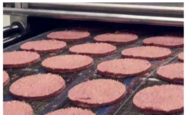
Burger patties approaching the X39 x-ray inspection system
