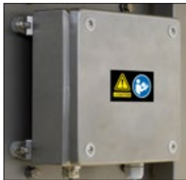
FIM enclosure box mounted onto the conveyor
