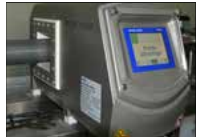
Profile Advantage systems overcome the issue of bubbles and voids in the product flow to virtually eliminate false rejects.
