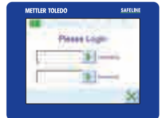
Dedicated 21 CFR part 11 mode with dual-level user name and password access login
