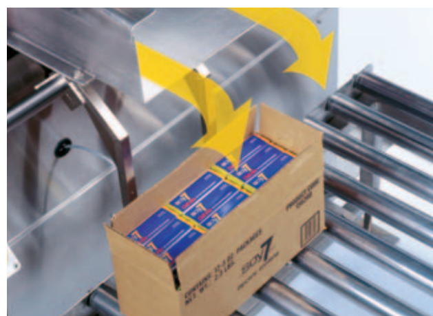
Loaded case is pneumatically lowered for discharge
