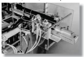
4. The side joint (flap) is glued just prior to right angle discharge of completed package.
