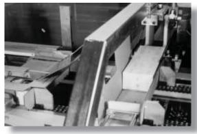
2. Product is loaded by optional automatic device (as shown) or manually.
