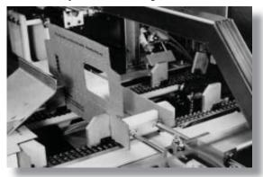
1. Partially formed blank is erected and transported to single product load station.
