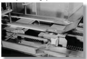
3. The package is then wrapped around the product and the end flaps are closed/sealed.
