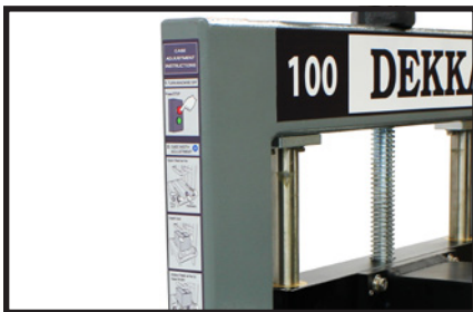
Color coded size change labels with pictorial guides
