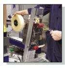
**Tilt-out Tape Head** Minimize downtime with the easily accessed bottom tape head, for fast tape changes. The tilt-out feature is exclusive to DEKKA tape heads.
