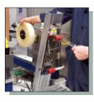
**Tilt-out Tape Head** Minimize downtime with the easily accessed bottom tape head, for fast tape changes. The automatic tilt-out feature is exclusive to DEKKA tapeheads. (Tape version only)
