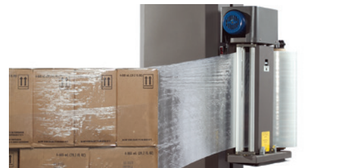
The film carriage prestretches film 200% prior to wrapping. This reduces material costs and strengthens the film for a tighter and more secure wrap. The machine E-stops if carriage detects an obstacle.
