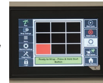
The Flex RT Series uses the IntelleVue operator touch panel to allow for easy programming of common settings. Advanced programming functions are password protected.
