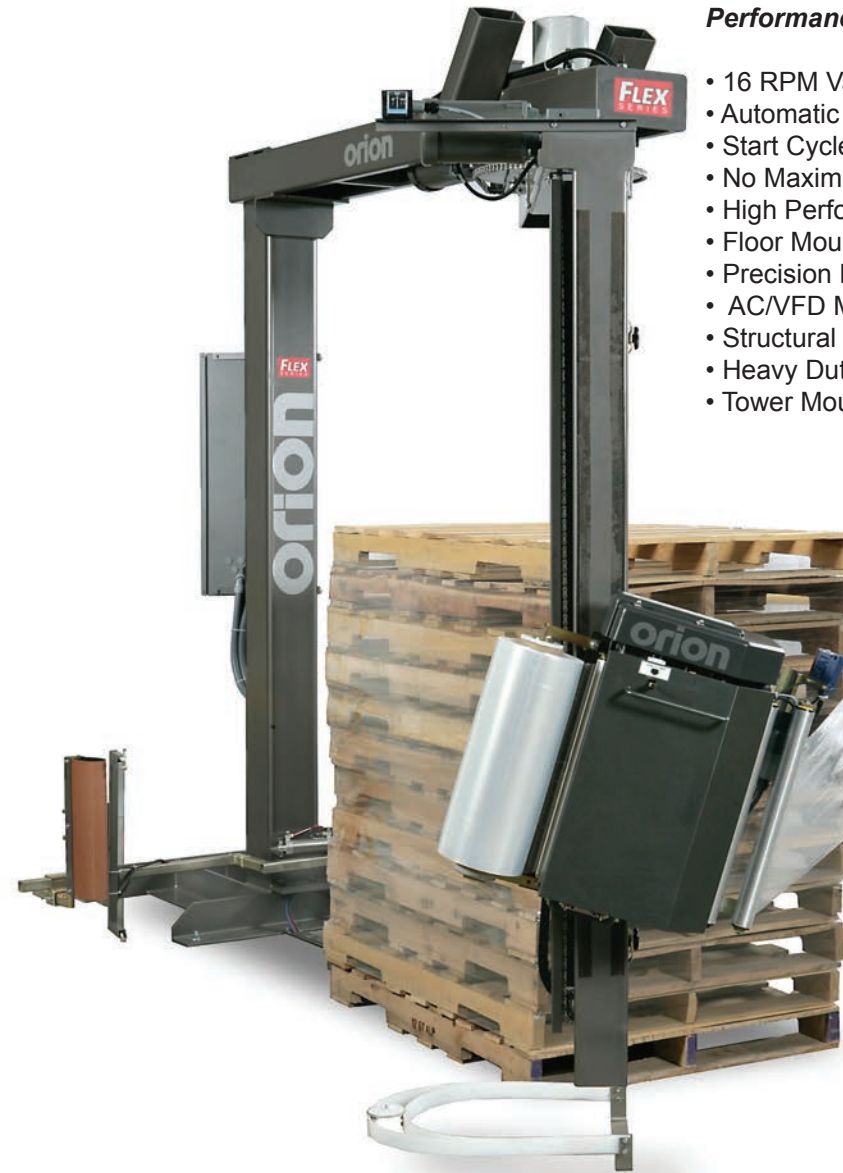
At the end of the wrapping cycle, Orion's innovative asymmetrical film clamp grips the film web while the impulse wire cuts the film. The load seeking brush then presses the film tail to the side of the load.
