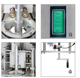
1. **Smooth and Even Film Cutting** The single-blade centrifugal cutting mechanism provides smooth and even cutting at high speeds
