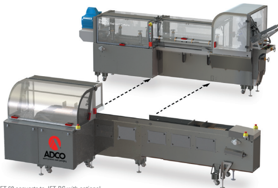
* JET-60 converts to JET-BC with optional auto-load barrel cam conversion shown here
