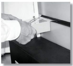
Operator presents one end of a carton in position over the glue pot and starts the cycle via a foot pedal.
