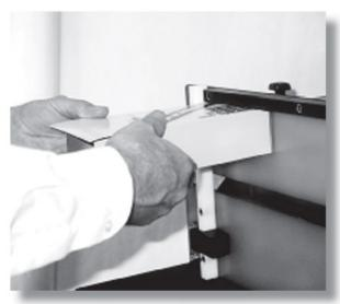
Carton is then manually lifted against a squaring device on the compression panel and hot melt seals the carton flaps.
